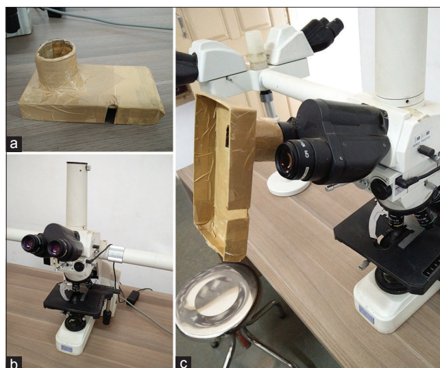
Figure 1: (a) Mobile phone mount made of the cardboard. (b) Nikon microscope. (c) Mount attached to the eye-piece of microscope
