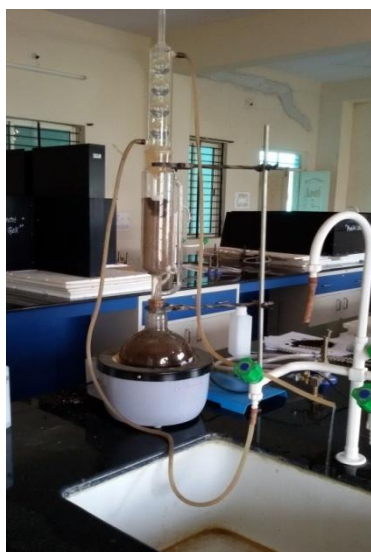
Extraction of drugs by Soxhlet apparatus
