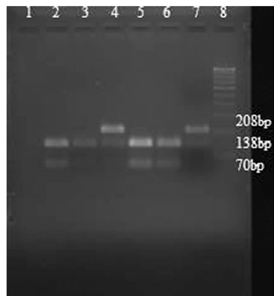
Fig. 2. Restriction analysis of H63D SNP after digestion with MboI. Lane no: 1 Negative control, Lane no: 2–7 autistic samples (Lane no: 2,3,5,6 was homozygote H/H allele. Lane no: 4, 7 was heterozygote H/D allele), Lane no: 8 marker 100 bp.
