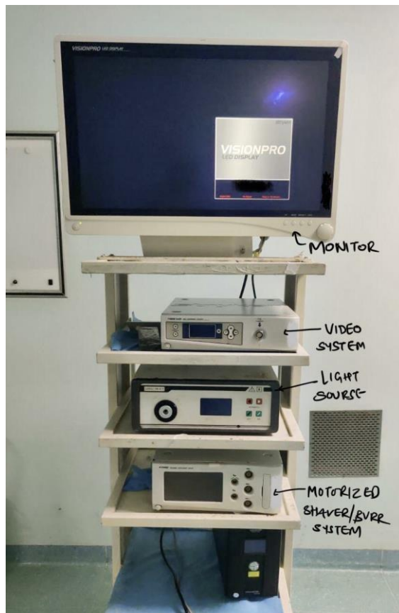
Fig 19: Trolley with video, light and motorized device system
