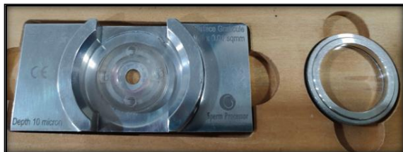
Figure 1: Makler chamber- Left -Base; Right- cover glass with metal ring
