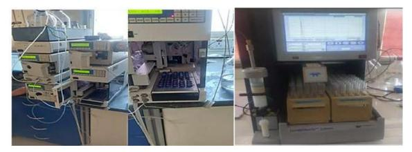
**Fig.3.** Instrumentation used for phytochemical analysis: (A) JASCO HPLC Autosampler for quantification of gallic acid; (B) Combi Flash RF+ Lumen system for purification of bioactive compounds.
