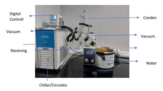
Figure No.4.12.1 Rotary evaporator
