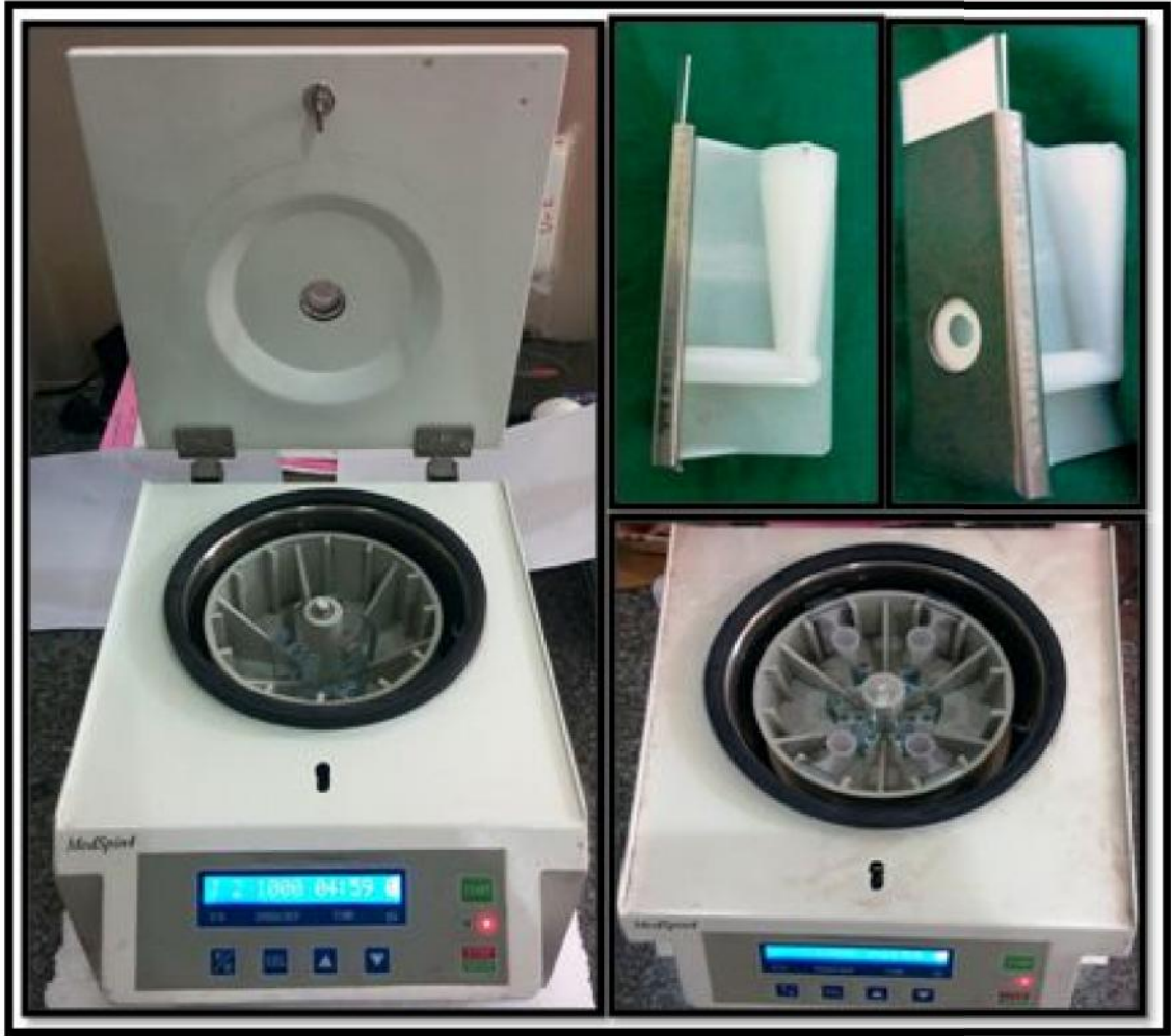
Figure 4.1: Cytospin(Med Spin 4) and Cytofunnel
